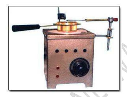
FLASH POINT AND FIRE POINT APPARATUS
